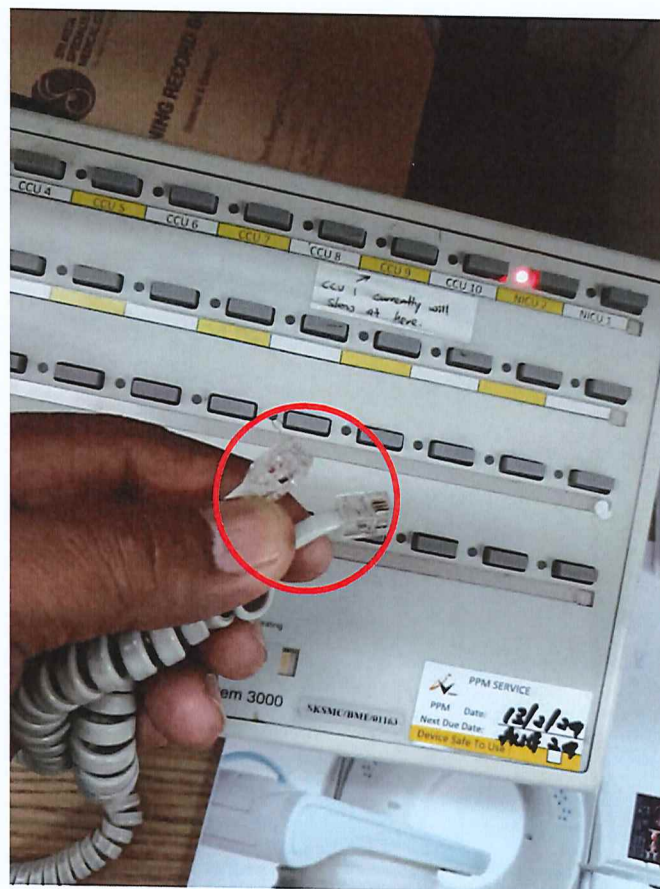
Patch Cord Cable for Console Found Faulty.
